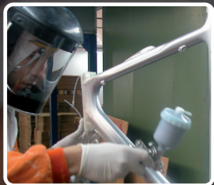
Special "mini" spray gun for maximum precision jobs.
