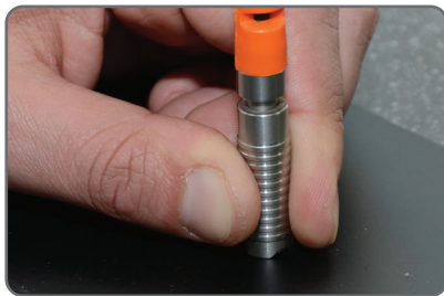
Probe Modules accurate to \pm 1\% or 1\mu\text{m} , whichever is the greater
