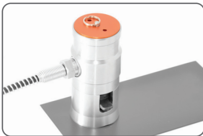
Quick connect coupling for 14.2, 20 and 50mm diameter dollies
