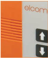
The speaker on the gauge clearly emits a ticking noise to indicate that there is voltage at the handle.
