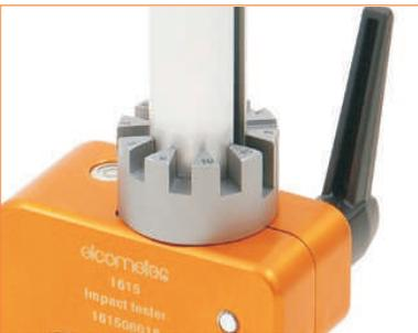
The stop collar, supplied with Kits A, D and F or as an optional accessory, allows the penetration depth to be limited. By rotating the stop collar, the user can select the depth required between 2 - 15mm (0.08 - 0.60").
