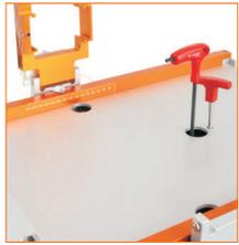
Stroke length can be adjusted by the user to meet specific requirements, from 10 to 300mm (0.4 to 11.8")
