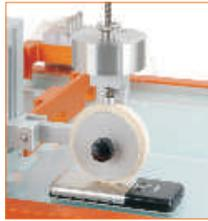
The rapid tool change system allows the user to test the samples in accordance with a wide range of National and International Standards on both flat and curved samples simultaneously
