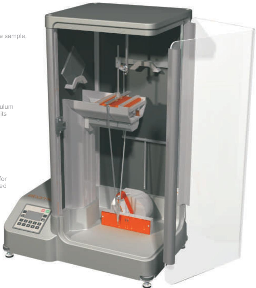
The hardness of any given coating is given by the number of oscillations within the specified limits of amplitude. The Persoz test measures the time taken for the amplitude of oscillations to decrease from 12° to 4°, whereas the König measures from 6° to 3°.
