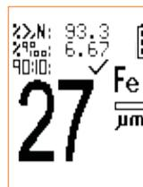
Provides the user with continuous monitoring of the 90/10 rule against the NDFT value, including pass/fail confirmation, as required by IMO PSPC for dedicated seawater ballast tanks.
