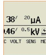
Adjust voltage via keypad on the gauge, with no need for screwdrivers. Sensitivity to current can be manually preset or automatically adjusted by the gauge for partially conductive coatings.
