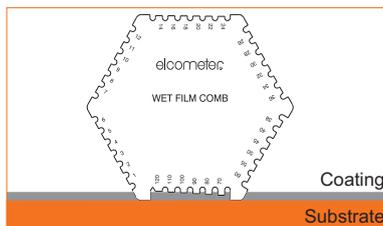
Place a comb perpendicular to and touching the substrate. Hold the comb in position and wait a few seconds until the teeth are wet. Remove the comb from the film.
