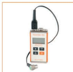
◀ Elcometer 204 Steel Ultrasonic Gauge, page 128
