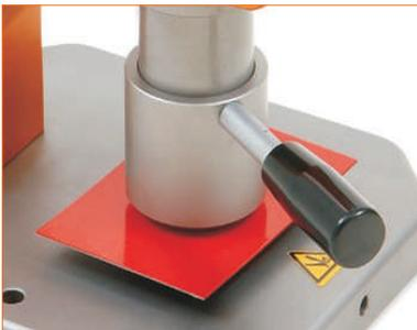
The Elcometer 1615 Variable Impact Testers are designed to meet a wide range of National and International Standards. Simply select the appropriate kit from pages 104 - 105 and attach the punch, die and accessories to the base unit. Interchangeable die - enables the user to match the die to the size of the relevant punch to conform to the required Standard or method.
