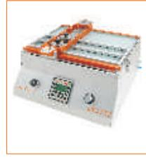
Stroke speed can be varied between 10 and 65 cycles/min or set to 37 cycles/min to meet ISO Standards
