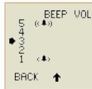
A loud audible alarm is activated when a spark is detected. The beep volume can also be adjusted to ensure it can be heard - even in noisy environments.
