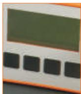
Large, backlit display enables easy viewing even in dark environments. When a flaw is detected the backlight also flashes.
