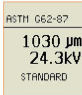
No need to use look up tables with the integrated voltage calculator. Enter the test standard and the coating thickness and the gauge will automatically programme the correct voltage.
