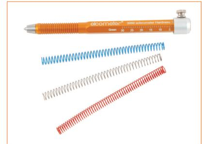
The spring force can be set by the “collar”; compressing the spring increases the force with which the tip is pushed on to the surface of the test piece. By making short, straight movements while gradually increasing the load, the user can observe the force at which the tip leaves a mark or destroys the coating.
