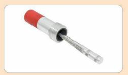
A small increase in the nozzle size will result in a very large increase in air and abrasive consumption and adversely affect blasting efficiency. To ensure your nozzle provides continuous high production, it is recommended, replacing your nozzle when the orifice wears by 1 nozzle size, when a #2 nozzle becomes the size of a #3 nozzle, for example.
