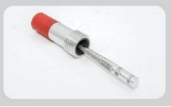
A small increase in the nozzle size will result in a very large increase in air and abrasive consumption and adversely affect blasting efficiency. To ensure your nozzle provides continuous high production, as a general rule, replace your nozzle when the orifice wears by 1 nozzle size, when a #2 nozzle becomes the size of a #3 nozzle, for example.
