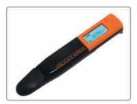
Incorporating a flat sensor, the Elcometer 138 Bresle Salt Meter measures the conductivity of a sample, then automatically converts this to show the density of salts, negating the need for the user to do a manual calculation when working in accordance with ISO 8502-6 or ISO 8502-9.
