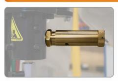
Pressure relief valves must be incorporated into the blast machine system to meet global safety standards. Elcometer's certified pressure relief valves can be easily fitted to the air manifold which is fitted to the RCV4000+remote control valve. Pressure relief valves are designed to discharge the compressed air in the blast machine upon reaching the crack pressure.
