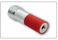
Featuring a liner made from hot-pressed boron carbide, this nozzle offers chemical and wear resistance properties, making it ideal for abrasives such as garnet, aluminium oxide and steel grit. As well as being heat and corrosion resistant, the nozzle's aluminium jacket makes it lightweight and its rubber sleeve is shock absorbent, preserving the internal liner. The nozzles are supplied with a rubber gasket.
