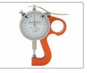
The Elcometer 124 Thickness Gauge is used to measure the peak-to-valley height of a surface profile moulded in the Elcometer 122 Testex® Replica Tape (page 9-9).
