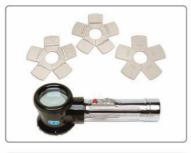
The Elcometer 127 range of Surface Comparators are available in sand, shot or grit surface profiles. Each comparator is supplied with 5 profile grades ranging from 0.5 - 5.5mils. Designed for use with the Elcometer 127 illuminated magnifier, each comparator has a hole in the centre allowing for clear visual comparisons to be made.
