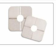
These extremely durable comparators allow the estimation of surface profile of either grit or shot blasted surfaces. Using the Elcometer 125 Surface Comparators as a reference the blasted profile can be compared to the four reference profile grades in each comparator. Profiles are recorded in microns.
