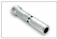
This nozzle offers a 35% larger blast pattern than a standard Venturi nozzle with only a small loss in abrasive velocity. Designed to be used on jobs where a more even dispersion of abrasive is required through a larger blast pattern. Supplied with a rubber gasket, it is ideally suited for use with plastic and cereal type abrasive media.
