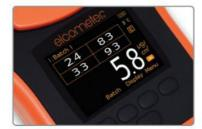
Four Bresle Patch Equivalent Readings
