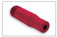
Designed to be hard wearing and long lasting, these blast nozzles feature a silicon nitride liner which reduces nozzle weight by approximately 50%. Supplied with a rubber gasket, the nozzle offers high temperature resistant properties, making it resistant to corrosion by many acids and alkalis. The acetal jacket also offers improved impact protection.
