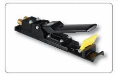
The B-Type Pneumatic Remote Control Handle, also referred to as a 'deadman's handle' is connected to the remote control valve using a twinline remote control hose and fastened to the blast nozzle allowing you to safely activate/deactivate the blast machine remotely.
