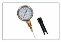
The Elcometer 102 Needle Pressure Gauge is designed to measure air pressure up to 20bar (300psi) in blast and air hoses. Pressure drop is responsible for decreased production rates, increased abrasive consumption and reduced anchor profile in abrasive blasting systems.
