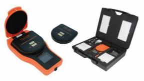
A Calibration Verification Tile is available for verifying the accuracy of the gauge whilst out in the field and the verification date is recorded for use in reports.
