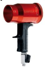
The Sagola Super Flow Drying Gun is a lightweight and practical tool designed to reduce drying time for waterborne paints. It features an adjustable venturi regulator for customized drying techniques, delivering up to 6,000l/min of air output to quickly evaporate water and speed up drying. The gun can be fully dismantled for easy cleaning and maintenance, while its heavy-duty construction ensures long service life.
