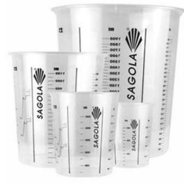
Made of polypropylene (PP5), high breaking thermal and chemical strength, the Sagola Mixing Cups are suitable for all paints. Four sizes are available to suit every need, all of them with feet to prevent spills by sticking to the table. Reinforced upper border for safe handling once filled, even in the largest size. Outer silkscreened high quality and solvent resistant.
