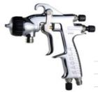
This Sagola 3300 GTO Pressure Spray Gun is supplied with a 1.20mm needle & nozzle size and GTO HVLP aircap, ideal for use with basecoats.
