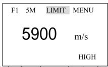
2) Press Enter display the low and high limit of previous setting (as shown in the figure), use  $\land$  or  $\lor$  to set the new low or high limit.
