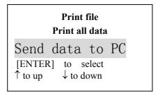
4) Press Enter confirm Send data, the screen will display: Send data to PC. When the sending is completed, the buzzer will give out sound, and the display will return to MENU state, and the display for that is:
