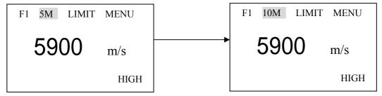
Each time you press ENTER, it will display in sequence the probe frequency to be set 2M (2MHz), 5M(5MHz) or 10M(10MHz).
