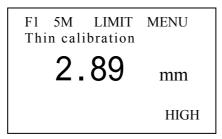
2) Measure the thinner standard test piece, use  $\land$  or  $\lor$  to adjust the measurement to standard value. Press ENTER, the screen prompts to measure the thicker piece, the display is as follows:
