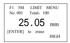
*Note*: **No.** is the serial number of the saved data displayed at present; **Total** is the total number of data saved in the file.
