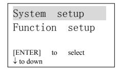
3) Press Enter enter System setup menu, press Enter display METRIC and IMPERIAL :
