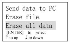
8) Press Enter confirm Erase all data, when the deletion is completed, the buzzer will give out sound, and the display will return to MENU state. The display for Erase is as follows:
