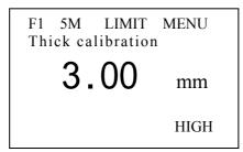
3) Measure the thicker standard test piece, use  $\land$  or  $\lor$  to adjust the measurement to standard value. Press ENTER, the calibration operation is finished.
