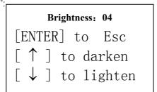
4) Use  $\land$  or  $\lor$  to adjust the display brightness, and exit setup by using **ENTER**
