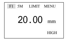
2) Press ENTER, by pressing F1~F5 to display file No.s cyclically. You can exit by pressing VEL or conducting one measurement. After setting file No., you can save the measured values into the file every time after you finished the measurement by pressing MEM.
