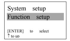
2) Press Enter to enter into Function setup, use  $\land$  or  $\lor$  to move cursor to Set brightness:
