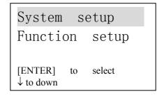
1) Press  $\vee$  to move the cursor to Function setup, the display is as follows:
