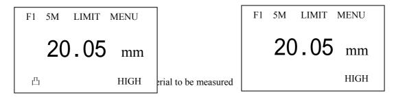
*Note*: when the probe is coupled with the material to be measured, the instrument will display the coupling indicator; if the indicator flashes or doesn't appear, it means that the coupling is not so good.
