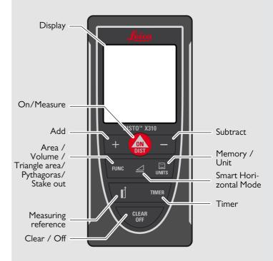
Instrument Set-up EN
