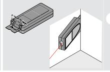
The orientation of the endpiece is automatically detected and the zero point is accordingly adjusted.
