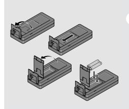
To ensure a reliable use, do not use zinc-carbon batteries.
