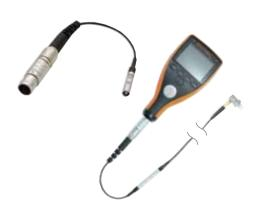
Simply plug the adaptor into the transducer connection point at the base of the gauge to connect any 'non-intelligent', single element transducer and follow the on-screen instructions.
