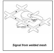
If the search head is held with the handle vertical, and scanned vertically between vertical bars, the maximum signal occurs every time the search head is over a horizontal bar. Similarly, with the handle horizontal, scanning sideways between the horizontal bars gives the maximum signal at each vertical bar.
