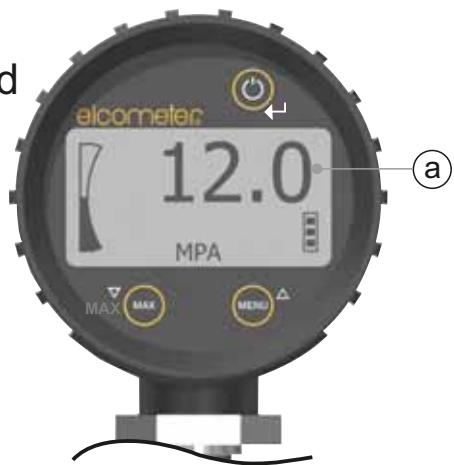
2 Record the pressure indicated on the display (a) and unwind the crank handle and coarse adjustment screw.
