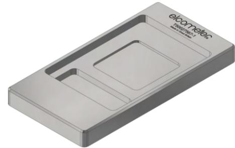
By using the Elcometer 500 CCM following the procedure outlined below, the Elcometer 500 gauge calibration will be traceable to National and International Standards.
