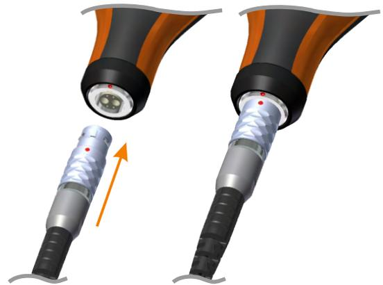
Elcometer 500 probes will be identified automatically by the gauge when connected and details can be viewed at any time via Menu/About/Probe Information.
