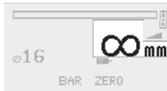
Figure 13. Depth of cover over-range (infinite)
