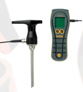
The Digital Balemaster is a handheld device with a large LCD display for easy reading. It features a robust stainless steel probe that is 558mm long and 10mm in diameter, designed to reach the center of large bales.
