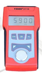
The TT2110 Ultrasonic Wall Material Thickness Gauge is a handheld, microprocessor-controlled device designed to measure the thickness of both metallic and non-metallic materials like steel, aluminum, titanium, ceramics, and glass. Includes a straight & right angle probe.
