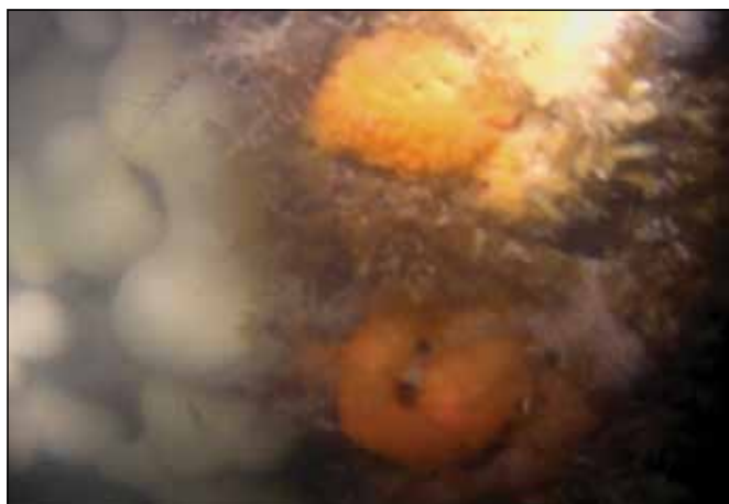
The corrosion cells/pits were covered with a bright orange plume with flakey, grey/black corrosion product underneath.
