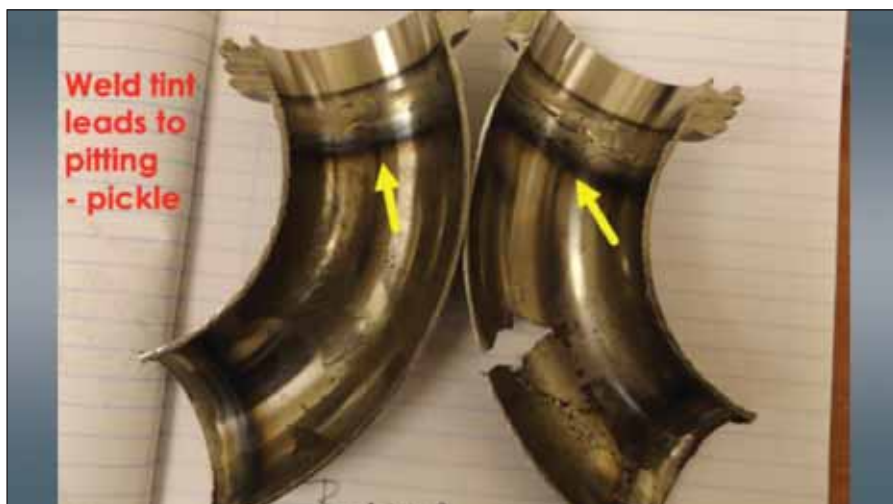
Figure 1 shows a 304L stainless steel pipe with dark heat tint which should have been pickled and has now shown pitting due to the heat tint oxide weakening the chromium oxide passive layer.
