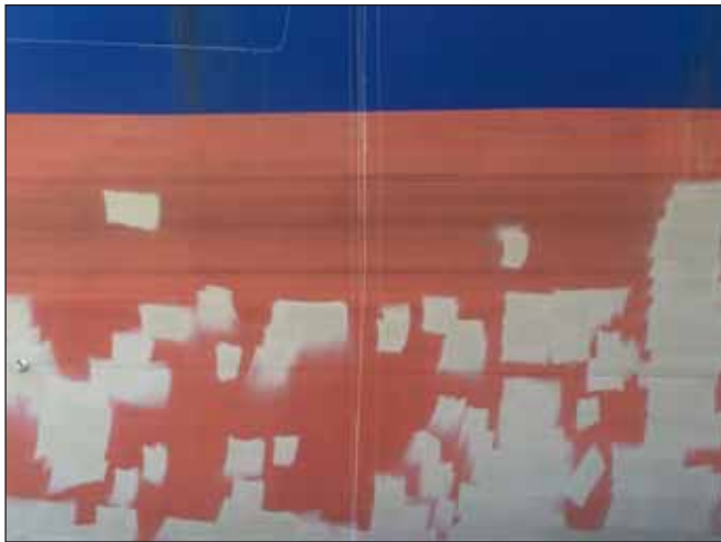
Tasport's Korimul Tug refurbishment over spot blasted surface with UHWJ.
