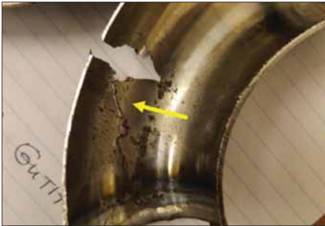
Figure 2: Stress corrosion cracking of a stainless steel pipe due to chloride containing fluid splashing on the outside of the pipe.
