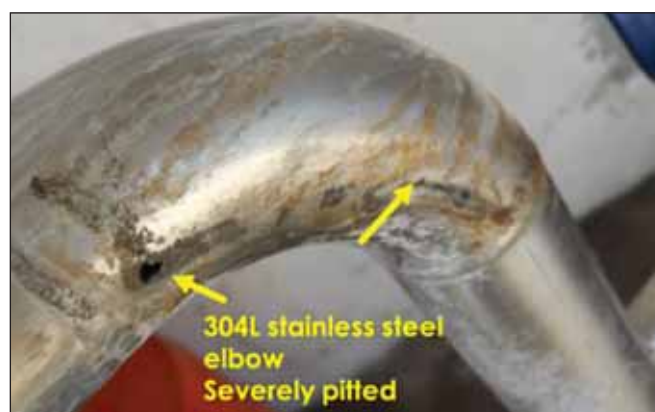
Figure 1: Pitting corrosion of a 304 stainless steel pipe at the weld seam.
