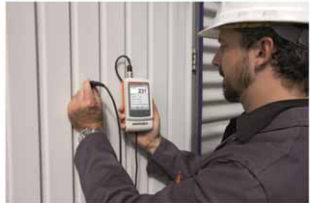
Fig. 2: Coating Thickness measurement with DUALSCOPE® FMP100
