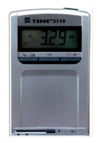
The TIME TR3110 is a portable surface roughness tester. It has a large measuring range suitable for most materials and has Ra and Rz parameters. It features an external calibration at the keyboard. The TR3110 is equipped with a Li-ion Battery.
