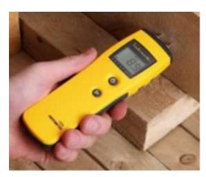
The Timbermaster is a new simple to use Digital moisture meter specifically designed for the timber industry. It is ideal for a range of quality control applications associated with the production, trading and use of wood products.
