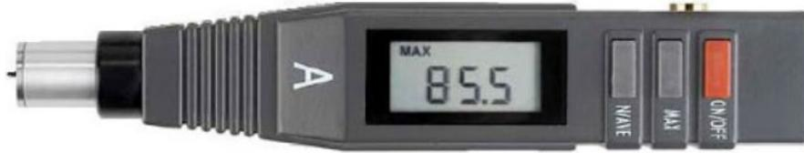
The TH200 Shore A Hardness Tester is a pocket-sized Digital Shore A Durometer for testing the material hardness of softer materials, including soft rubbers, plastics, silicone, leather, and printing rollers.
