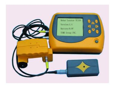
The TC110 is used to detect the thickness of concrete covering layer and rebar diameter. Besides, it can detect the location of magnetic substance and electric conductor in non-magnetic and non-conductive medium, e.g. cable inside wall body and water & heating pipe etc. It is a kind of intelligent nondestructive test equipment possessing the functions of automatic detection, data memory and output.
