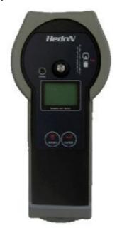
The Soluble Salt Meter (SSM) is developed specifically to address problems with US Navy and IMO test protocols using the Bresle Patch. The SSM exactly duplicates the Bresle Patch process but with a higher accuracy and reproducibility. Measurements are automated and there are no consumables. The complete test sequence requires less than a minute.
