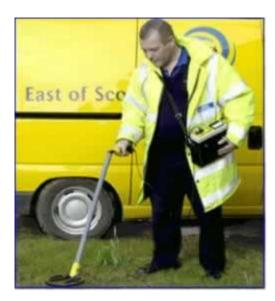
The Elcometer P520 Metal Detector is very high powered for greater depth detection. Originally designed to locate water mains, pipes and cables the Elcometer P520 is also the perfect choice for location work in cluttered areas and at depths where other metal detectors simply do not work.
