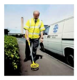
Although originally designed to accurately locate valve boxes and manhole covers, the Elcometer P500 can also be used as a general purpose metal detector. The Elcometer P500 is both deceptively simple to use and very rugged making it a favourite choice in the market.
