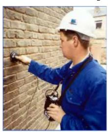
Having been approached by a contractor engaged in replacing wall ties, we designed an instrument specifically to identify the location of the wall ties. A product of this type has to be fast, stable and accurate. Require no zeroing, be easy to use and extremely tough.
