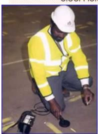
Rebar Plus concrete rebar locators are the easiest and fastest way of detecting reinforcing bars in concrete. It is widely used before coring or drilling holes to find "safe spots". It will indicate the rebar location and direction and will also give an indication of the depth of concrete cover.
