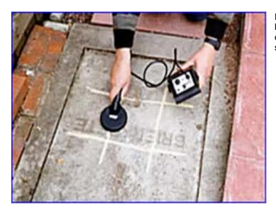
Robust and economical, the Imp concrete rebar locator is an ideal and versatile detector, it can also be extended to detect mild steel wall ties or even stainless steel and galvanised wall ties.
