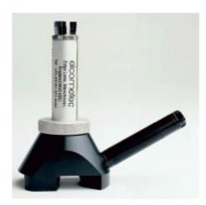
This very simple graduated x50 magnification microscope is an ideal gauge for measuring the size of cracks in concrete.
