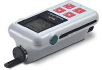
In protective coating applications there is a requirement to measure surface roughness.
