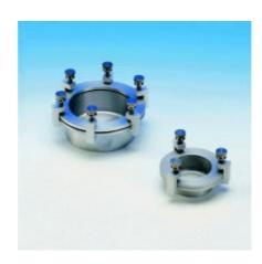
Instrument made entirely of anodised aluminium, used to determine the permeability of films of paint, varnish, plastic, cellophane, etc.
