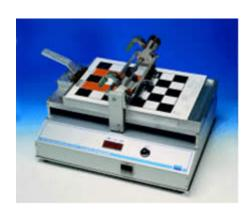
An essential machine for preparing a wide variety of product samples including: paint, varnish, cosmetics, glue, etc, with total consistency and reproducibility on various substrates including contrast charts, sheet steel, plastic foils and glass.
