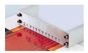
Made of stainless steel, the straight scraper has 10 adjacent notches of increasing clearance. The Elcometer 4270 Sag Tester is used to establish the coatings resistance to sag due to gravity.
