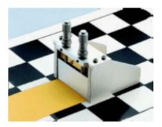
Manufactured in anodised aluminium, with a bevelled blade applicator body, the Elcometer 3580 is suitable for manually applying thick layers of various products, on solid and flat substrates.
