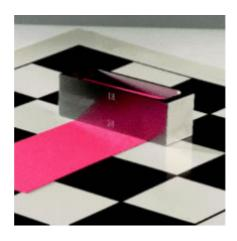
A simple gauge with a single reservoir allowing the user to generate 4 different thicknesses of coating.
