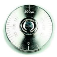
Stainless steel device, to measure the thickness of wet films
