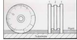
Roll the wheel through the wet film with the side 1 in the diagram touching the substrate. Roll for at least one whole turn and slowly enough for wetting to occur. Roll the wheel backwards by at least on complete turn. The wet film thickness is read from the scale, at the end of the wetted segment of the middle circle, 2 in the diagram
