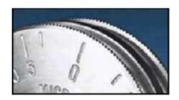
Similar to the Elcometer 3230 Wet film Wheels, but designed for use in the coil coating process. These Coil Coating Wheels consist of three circles. The outer circles are knurled to allow measurements to be taken on slippery coatings or on fast moving substrates.
