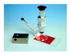
Unit for measuring hardness by the indentation of a bevelled disc indenting tool with a sharp edge. This is fitted onto a steel block with two supports providing a constant test load of 500g. When placed on a coating for 30 seconds, the disc leaves a trace that can be observed with the x20 microscope, with graduations every 0.1mm. The indentation length is then recorded. This length of the trace is inversely proportional to the hardness.
