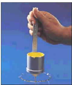
Thanks to its handle, this cup is very easy to use and performs quick controls in workshops or during the manufacturing process. Ideal for measuring the consistency of paints, varnishes and similar products.
