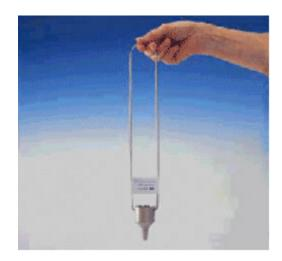
A stainless steel cup for quick measurements on-site or during production. This cup is often used in the printing or ink industry. The cup is first dipped into the product to be measured, then empties through the orifice.
