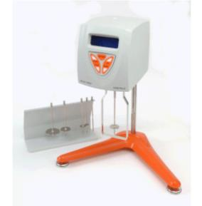
The Elcometer 2300 Rotational Viscometer range measures the viscosity of liquids in accordance with several standards. Using a rotational viscometer, the properties of liquids and their resistance to shear or flow can be accurately measured.
