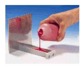
This simple instrument is used to assess the ability of thick or paste-like materials such as paints or printing inks to flow.
