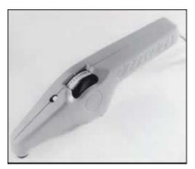
Coating thickness gauges are used in maintenance and periodical inspection as well as during the coating process.
