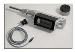
Test hammers are used to determine the surface hardness of concrete and are one of the most widely used instruments in the field of non destructive testing (NDT) of concrete compressive strength. It is the quickest, simplest and least expensive method to obtain an estimate of the quality and strength of the concrete.
