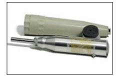
This simple to use gauge consists of a spring loaded plunger which, when released, strikes the surface with fixed and constant impact energy. During the rebound stroke, the mass moves a pointer that indicates the maximum point of return and at the same time indicates a reference value called Rebound Number.
