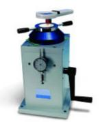
These robust and user-friendly instruments are used for assessing the cupping ability of coatings applied to metal sheets up to 1.2mm thick.
