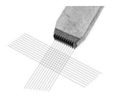
Simple instrument for quickly determining the adhesion of a large number of paints. Made from special steel, it has 11 tapered teeth with 1 mm spacing.
