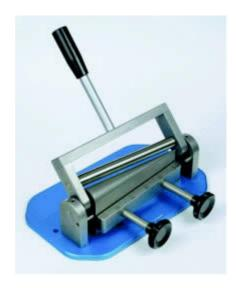
Mechanical testing equipment for the determination of elasticity, adhesion and elongation of paint on sheet metal. The frame has a bending lever with a roller which pivots on a steel conical mandrel with a diameter from 3.2 to 38.1mm. A graduation indicates the mandrel diameter in mm and inches.
