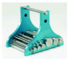
A simple instrument for determining the elasticity, adhesion and cracking of dry paint on flat specimens, consisting of a mandrel support which also serves as a test stand.
