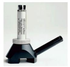
This very simple graduated x50 magnification microscope is an ideal gauge for measuring the size of cracks in concrete.
