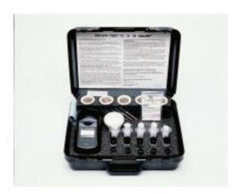
Designed to accurately measure surface chloride, sulphate and nitrate ions in minutes, the Elcometer 134 'CSN Salts' offers the user the ability of trouble-free performance testing in the field.
